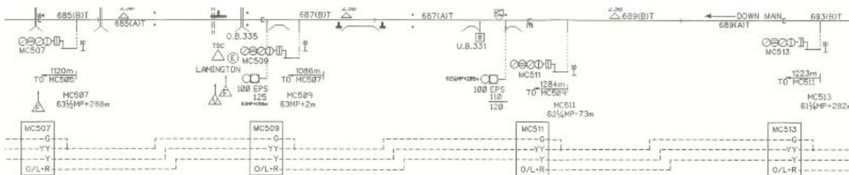
Technical Headway at Signal MC513 (above right) is the time elapse between the front of the first train passing MC513 (showing a green aspect) and its rear clearing the overlap of MC507 (above left), this being the point at which MC513 would be able to show a green aspect again. To this must be added a system reset time (normally 4s but this can vary) and sighting time for the second train to see MC513 at green (this is a standard 9s as used by signal sighting committees).
