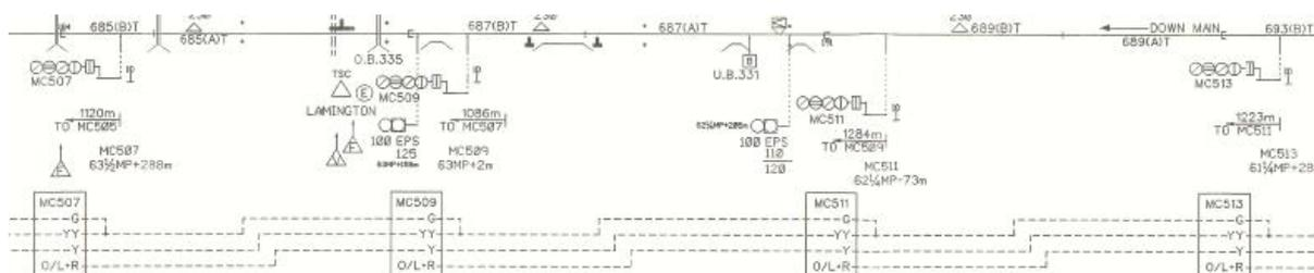
Technical Headway at Signal MC513 (above right) is the time elapse between the front of the first train passing MC513 (showing a green aspect) and its rear clearing the overlap of MC507 (above left), this being the point at which MC513 would be able to show a green aspect again. To this must be added a system reset time (**normally 4s but this can vary**) and sighting time for the second train to see MC513 at green (this is a standard 9s as used by signal sighting committees).
