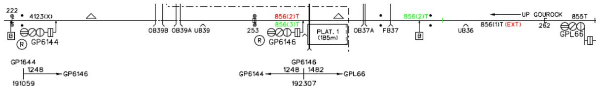
Technical Headway at Signal GPL66 (above right) is the time elapse between the front of the first train passing GPL66 (showing a green aspect) and its rear clearing the overlap of GP6144 (above left), this being the point at which GPL66 would be able to show a green aspect again. Again, to this must be added the system reset time and the sighting time for the second train to see GPL66 at green.
