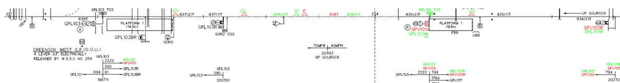
Technical Headway at Signal GPU105 (above centre-right) is the time elapse between the front of the first train passing GPU105 (showing a green aspect) and its rear clearing the overlap of GPL103 (above left), this being the point at which GPU105 would be able to show a green aspect again. Again, the system reset time and sighting time must be added.
