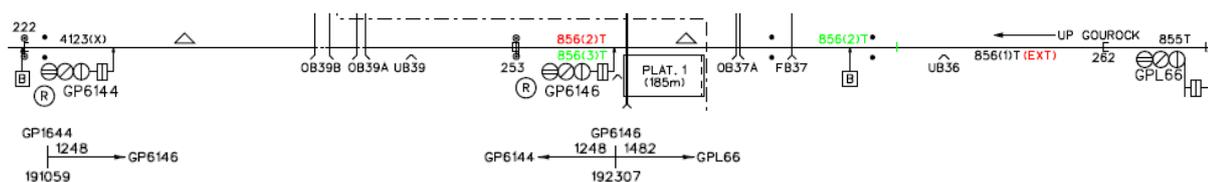
Technical Headway at Signal GPL66 (above right) is the time elapse between the front of the first train passing GPL66 (showing a green aspect) and its rear clearing the overlap of GP6144 (above left), this being the point at which GPL66 would be able to show a green aspect again. Again, to this must be added the system reset time and the sighting time for the second train to see GPL66 at green.
