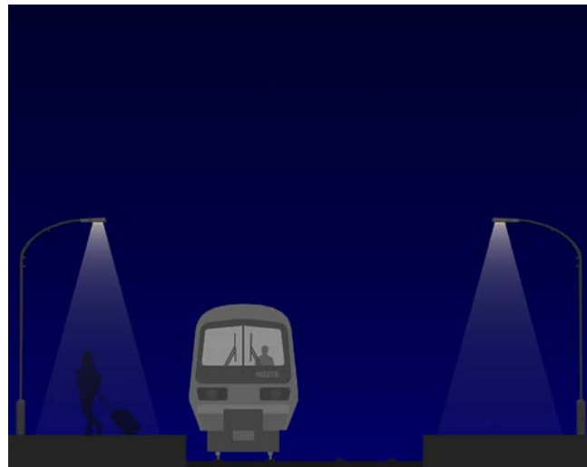
Figure 4.4 Column mounted luminaires illuminate open platform surfaces
