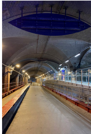
Image 4.52: Leeds Station High reflectance light coloured floor finishes create a sense of spaciousness.
