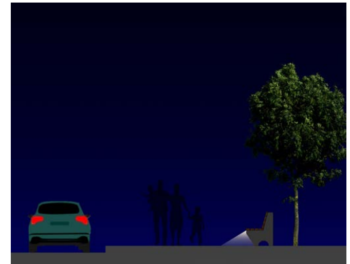
Figure 4.11 Low level lighting integrated into street furniture assists orientation.
