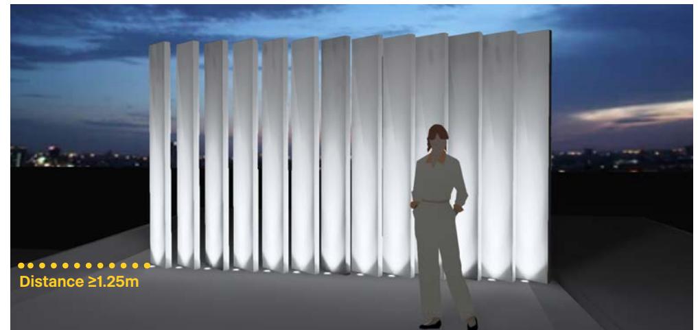
Figure 4.35: Possible design of the louvre screen
