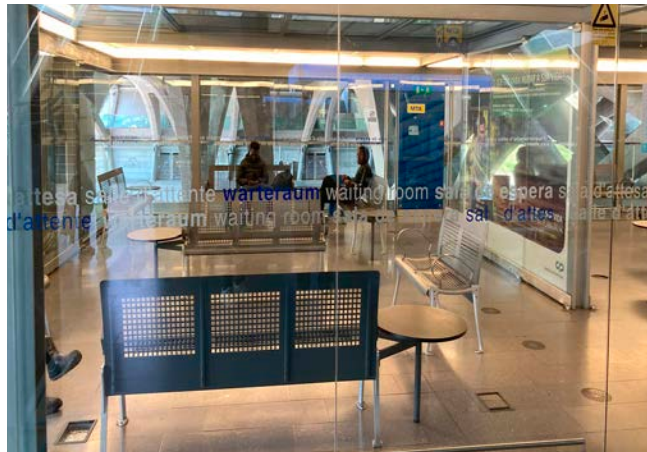
Image 4.68: Oriente Station, Lisbon Clear structural glass with manifestation creates a sheltered space.
