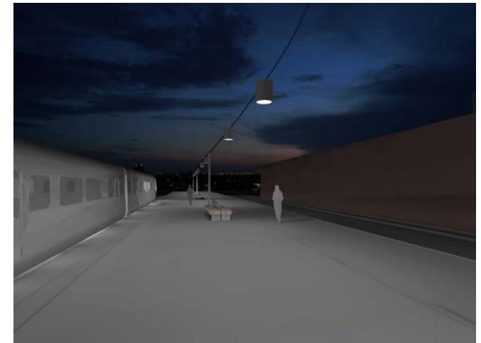
Figure 4.30: Catenary lighting installation suspended along centre line of the platform
