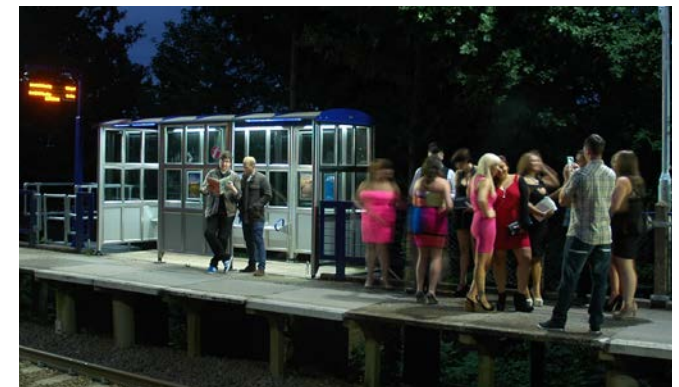
Image 4.71: Modular shelter with integrated lighting has higher levels of illuminance than the adjacent platform
