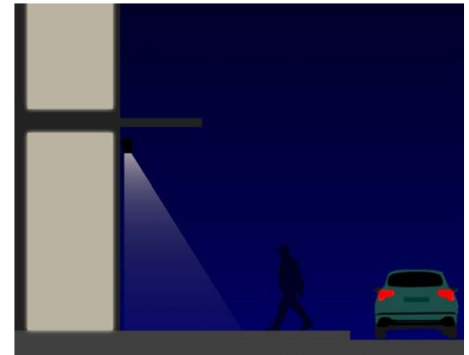
Figure 4.5 Wall mounted luminaires illuminate station forecourt
