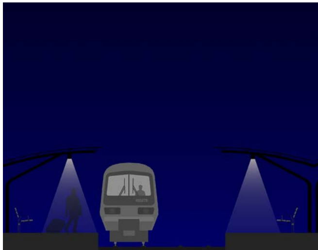
Figure 4.3 Linear luminaires mounted on continuous CMS beneath canopy
