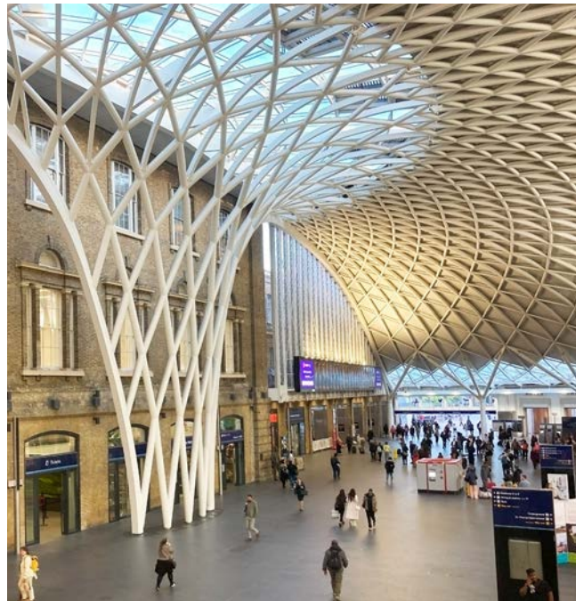
Image 2.22: Kings Cross Station Ambient lighting levels in the concourse area are carefully balanced with exterior daylight conditions, facilitating a smooth transition from the external public realm to the interior spaces of the station.
