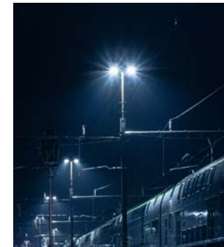
Image 2.24: Disability Glare from visible light sources on high masts.
