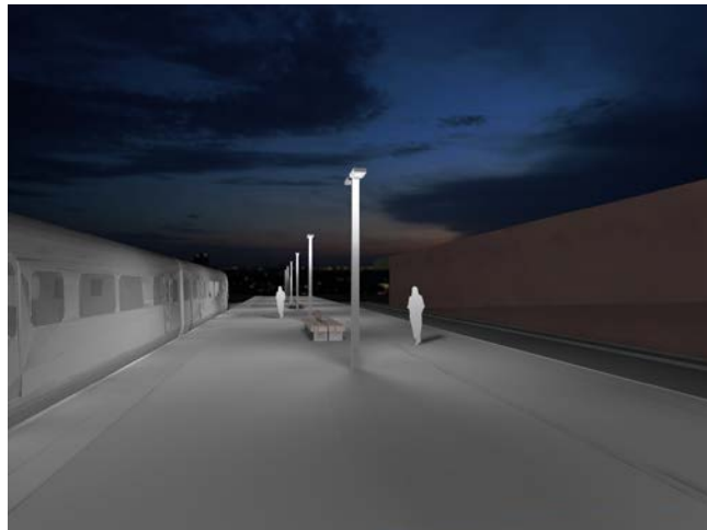
Figure 4.29: Typical twin headed lighting columns aligned with centre line of the platform
