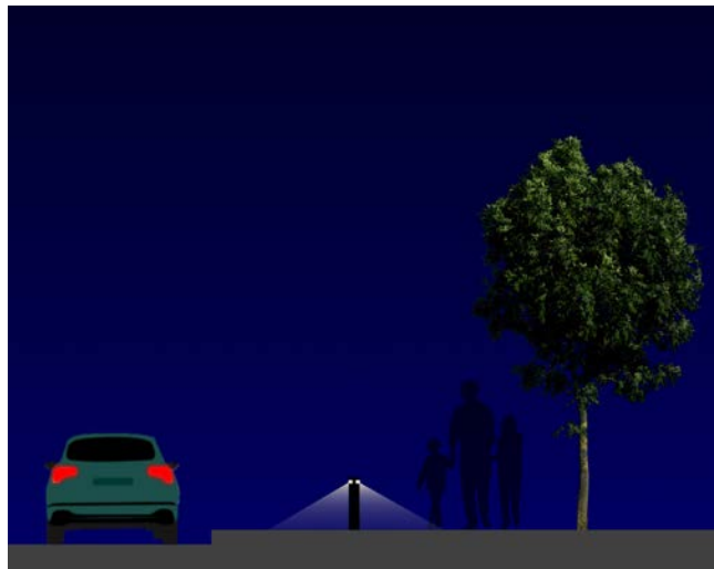
Figure 4.7 Illuminated bollard with shielded downward light distribution.
