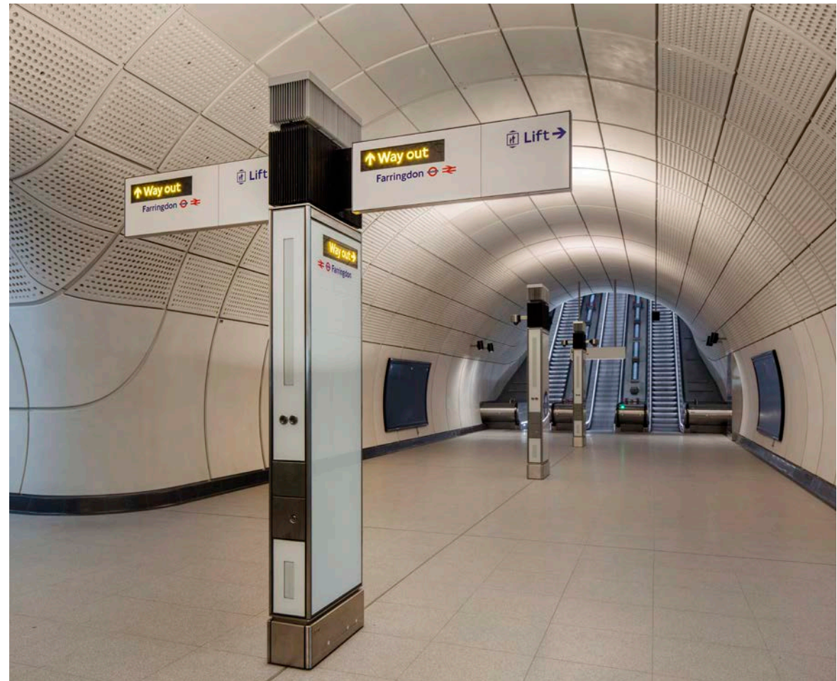
Image 2.14: Elizabeth Line concourse Lighting integrated in architectural elements. Uplighting creates a sense of elevated ceiling
