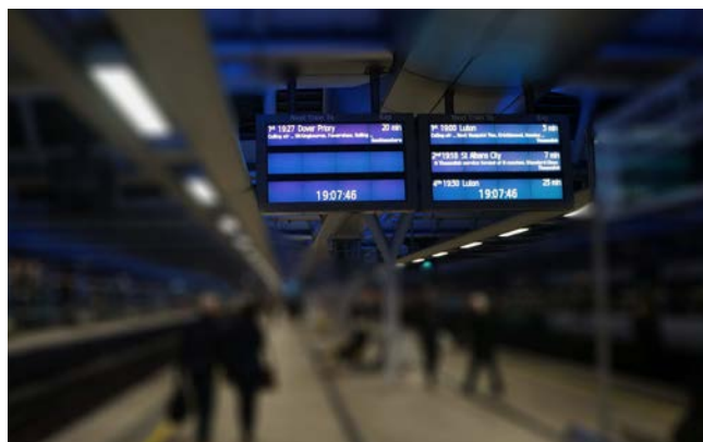
Image 2.19 Passengers with visual impairment may have difficulty reading Customer Information Displays. Platform surfaces with high reflectance values and good levels of illuminance with high levels of lighting uniformity can assist all user groups in the station environment.
