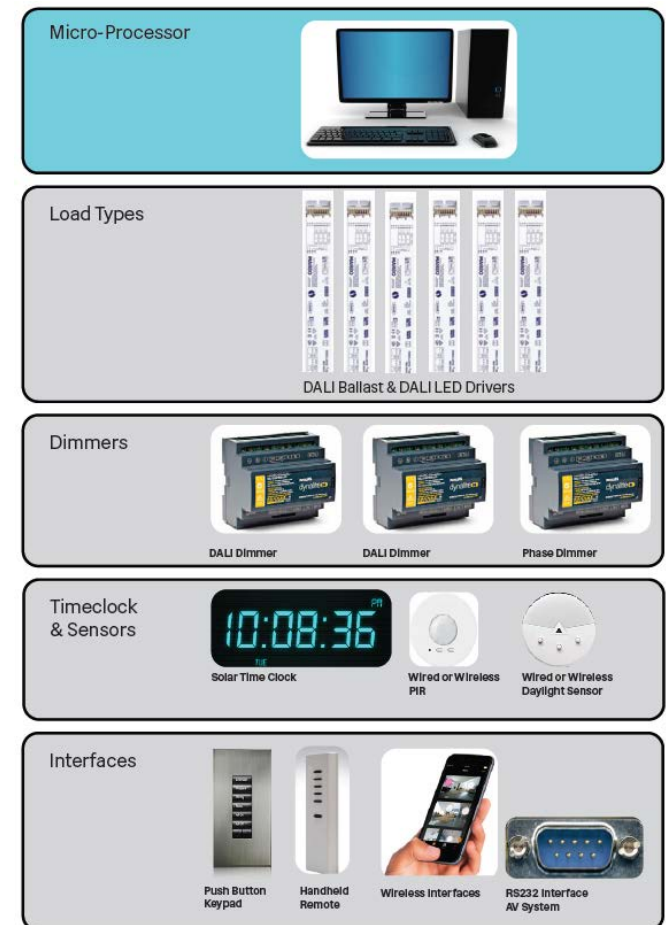
Figure 6.6: Typical control system architecture - indicative only
