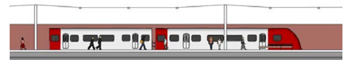
Figure 4.32: Proposed catenary lighting alternative. This solution has fewer lighting columns than a standard solution and offers the possibility of integrating other station services, such as CCTV, PAVA CIS etc. which usually require separate structures to be provided.
