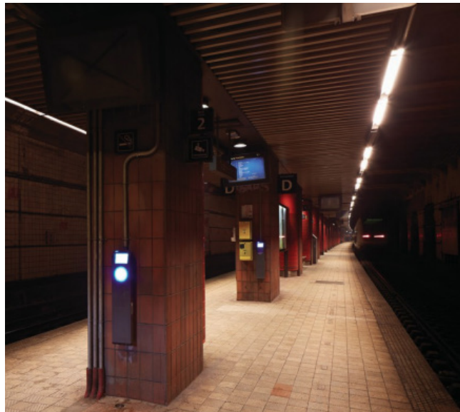
Image 8.6: The previous scheme at Nørreport Station. Dark surface finishes on the columns and ceiling combined with direct-only lighting scheme created a less inviting space for users.
