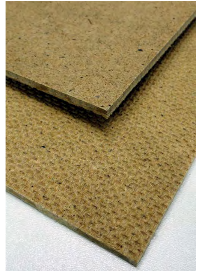
Image 2.13 Hardboard with smooth and mesh textures
