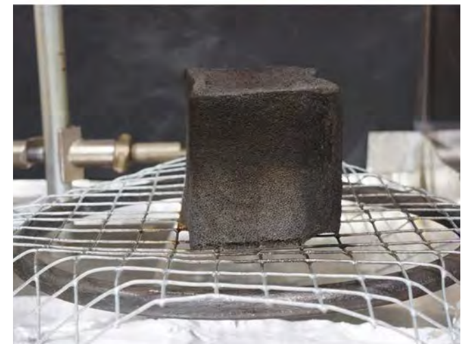
Image 1.37 Material fire certification testing
