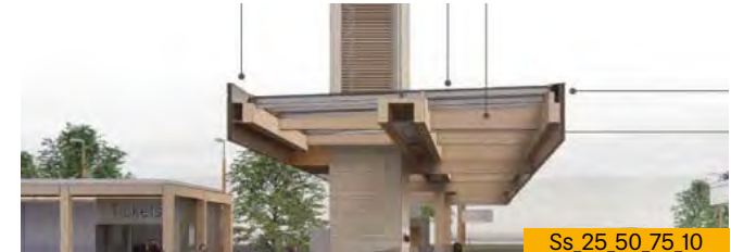
Free standing Cantilever - Glazed wind break
