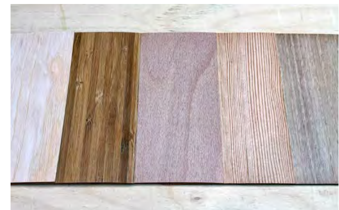
Image 2.20 Flexible wood veneer samples
